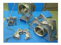
Where fast, easy and precise installation/removal of metallic bellows is needed, typically in series installation and preventive maintenance operations, the rapid bellow compression tool is used. This technique allows fast axial compression/expansion of bellows using two concentric articulated collars permitting quick opening and closing around the bellow.
