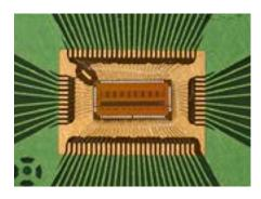
CERN has available a low power front-end amplifier discriminator ASIC chip for use in applications based on electron and photon detecting in medical imaging, life science or material research. This NINO ASIC allows for an 8-channel input signal charge measurement through encoding discriminator pulse width with excellent timing resolution at very high rate, while at the same time providing a very low noise performance and power consumption characteristics per channel.
