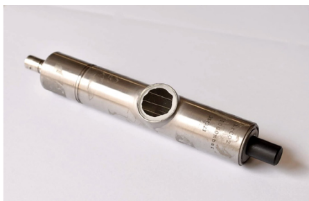
Supersensitive flame detector prototype based on wire amplification structure. (Image: CERN)
