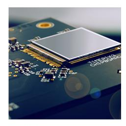
A pixel detector read-out chip for X-ray imaging and particle track reconstruction developed by the Medipix3 Collaboration.
