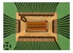
CERN has available a low power front-end amplifier discriminator ASIC chip for use in applications based on electron and photon detecting in medical imaging, life science or material research. This NINO ASIC allows for an 8-channel input signal charge measurement through encoding discriminator pulse width with excellent timing resolution at very high rate, while at the same time providing a very low noise performance and power consumption characteristics per channel.
