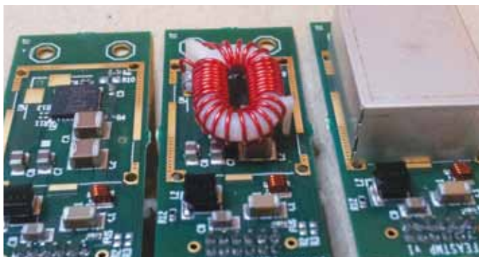
DC-DC plugin module holding the FEAST ASIC
