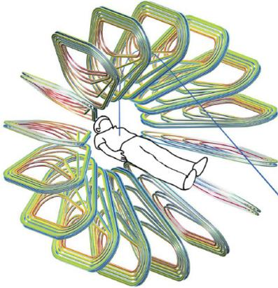
A compact and non-rotating gantry for charged particle therapy.
